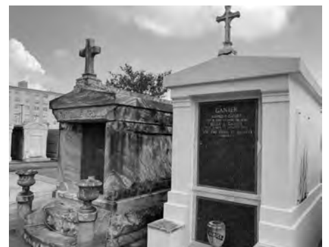
Due to the high water table, crypts are built above-ground.
